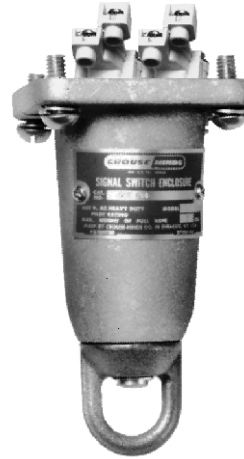
AFU mine signal switch with pushbutton switch (cover removed)
